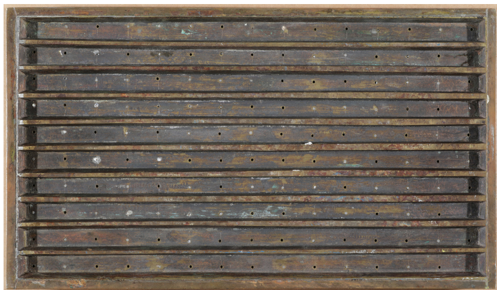
The reverse side of the plate. Each cliché was firmly mounted in the cradle by the means of a steel pin [photo: Ioannis Assimakopoulos, Athens].
